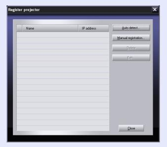
Use the "Registration using automatic detection" ( p.5) or "Registration using IP address (Manual registration)" ( p.6) procedure to register projectors.
